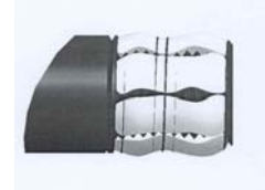
CAUTION: EXCESSIVE COMPOUND MAY BLOCK DISC OFF VALVE SEAT CAUSING LEAKS.
