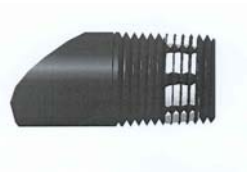
APPLY A MODERATE AMOUNT OF PIPE COMPOUND TO PIPE ONLY (LEAVE TWO END THREADS BARE).
